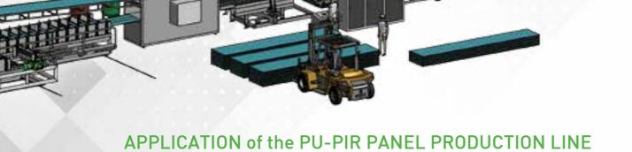
This production line is suitable for manufacturing socket type ( wall plate panel ) and lapped type ( roof tile panel ) pu sandwich panels.
